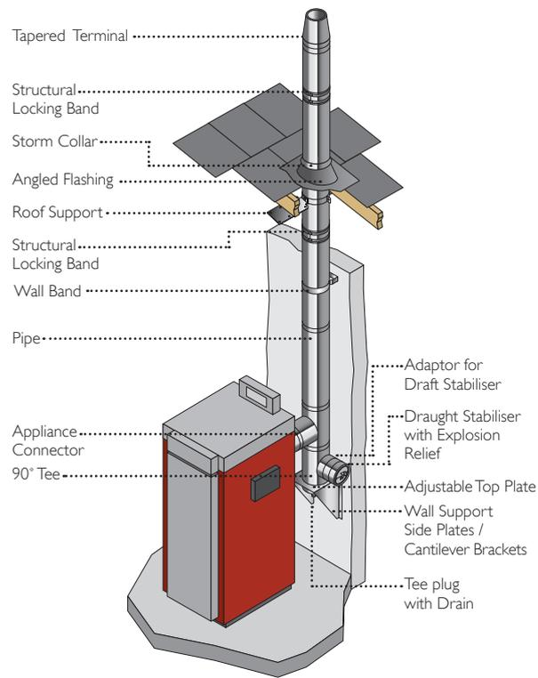
**TYPICAL BIOMASS INSTALLATION FROM REAR OUTLET USING ICS SYSTEM CHIMNEY WITH 90° TEE SOLUTION**
