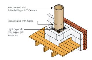
Clad the flue liners with a minimum of 100mm suitable masonry. A minimum of 15mm Leca insulation must be installed between the flue liners and masonry. Mix 20 parts Leca to 1 Part cement and a small amount of water. Ensure it is well mixed before using. (refer to table on page 3)
